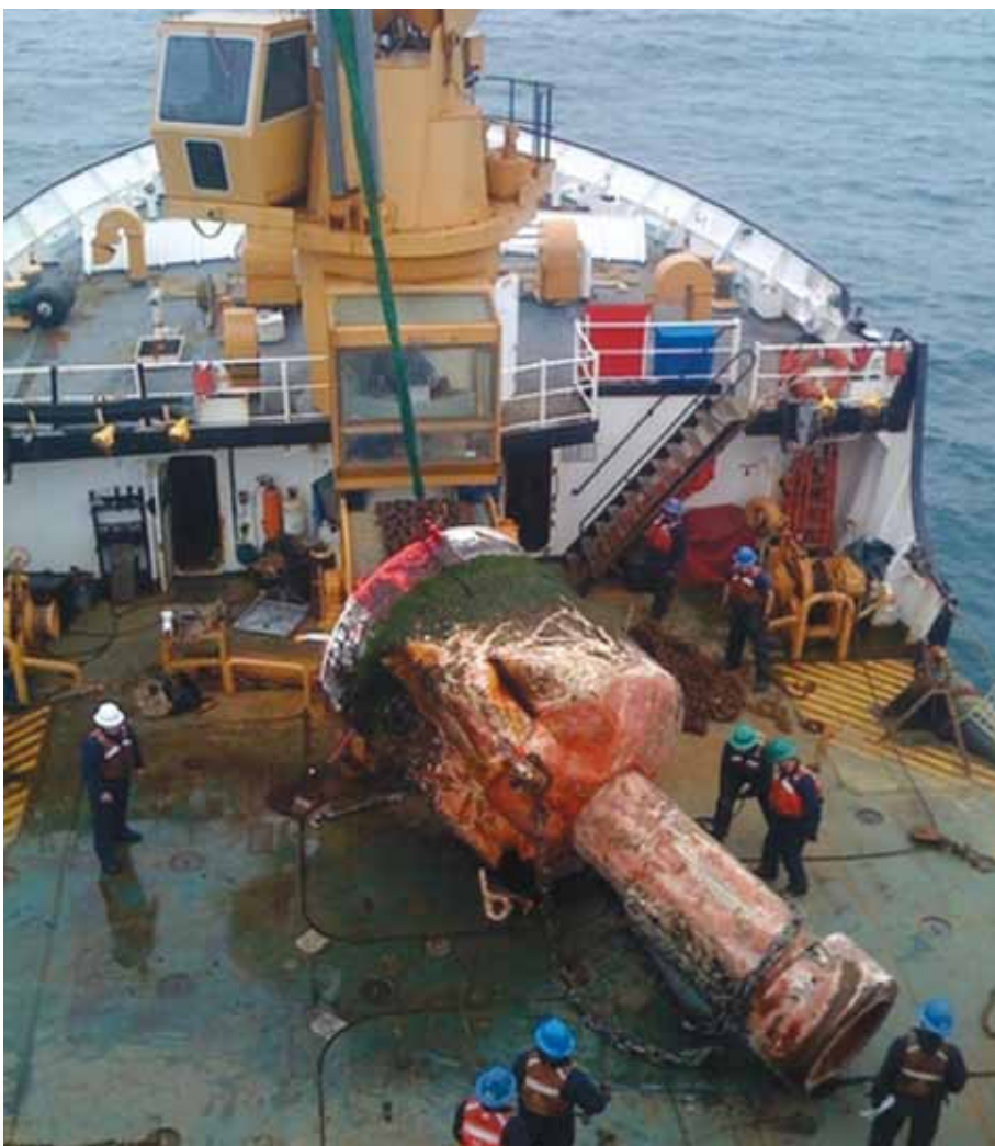
Crewmembers on the U.S. Coast Guard Cutter Aspen lower the San Francisco Approach Buoy onto the deck of the Cutter after retrieving it from the bottom of the water. The buoy was missing after an outbound ship reportedly struck it.
