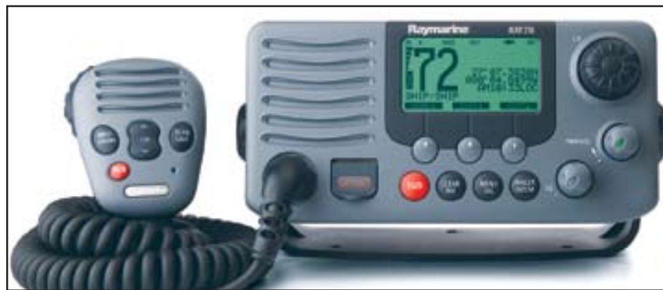
Fixed-mounted VHF with DSC capability.
