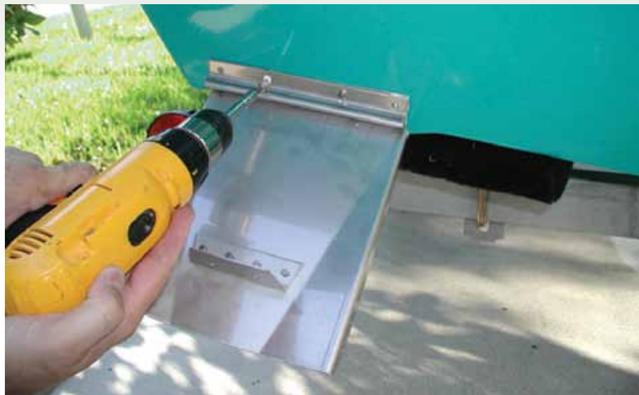
A trim tab is installed on the port side of the transom.
